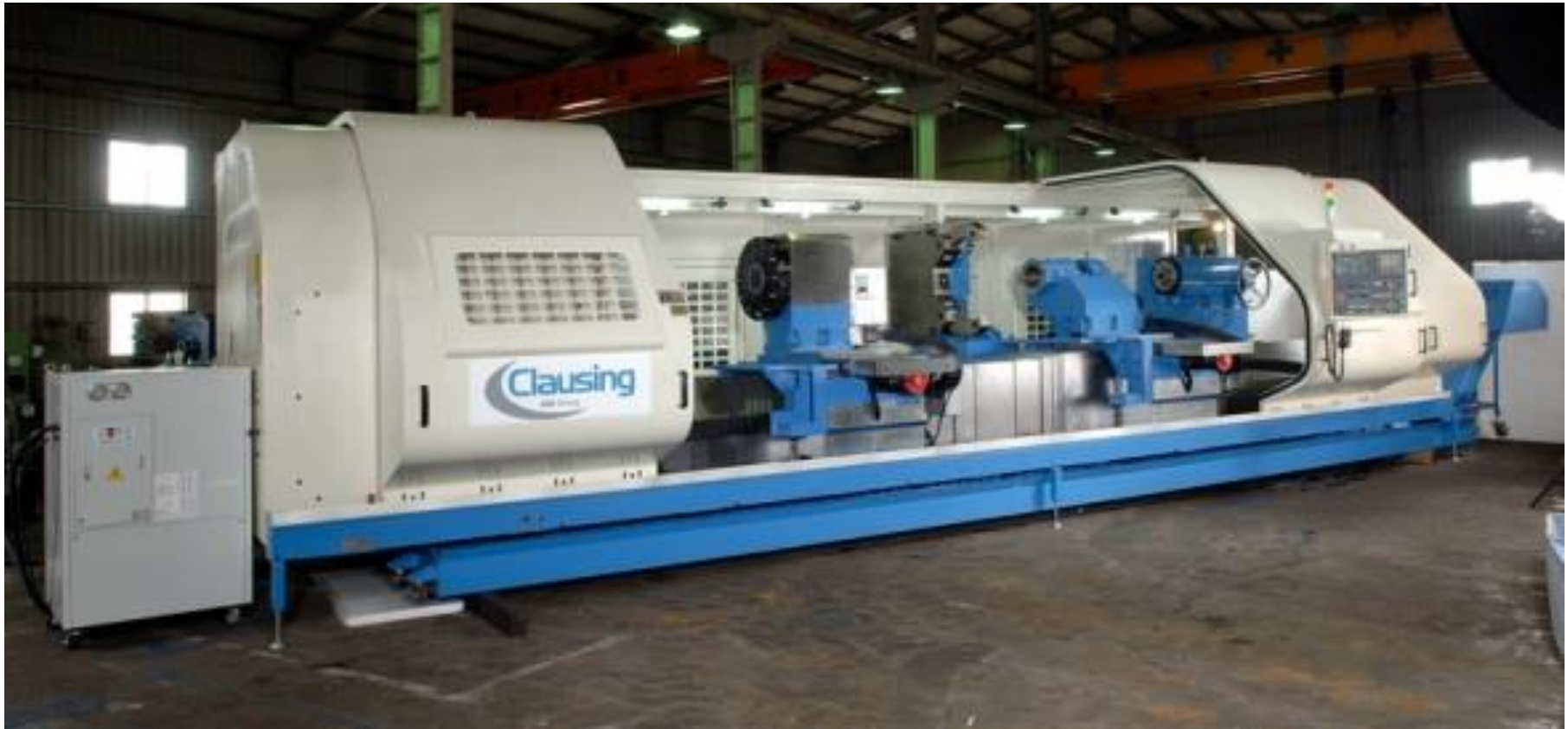
6 x 1.3 metre Large Swing Lathe, Installed at Halliburton (Malaysia) by Clausing
